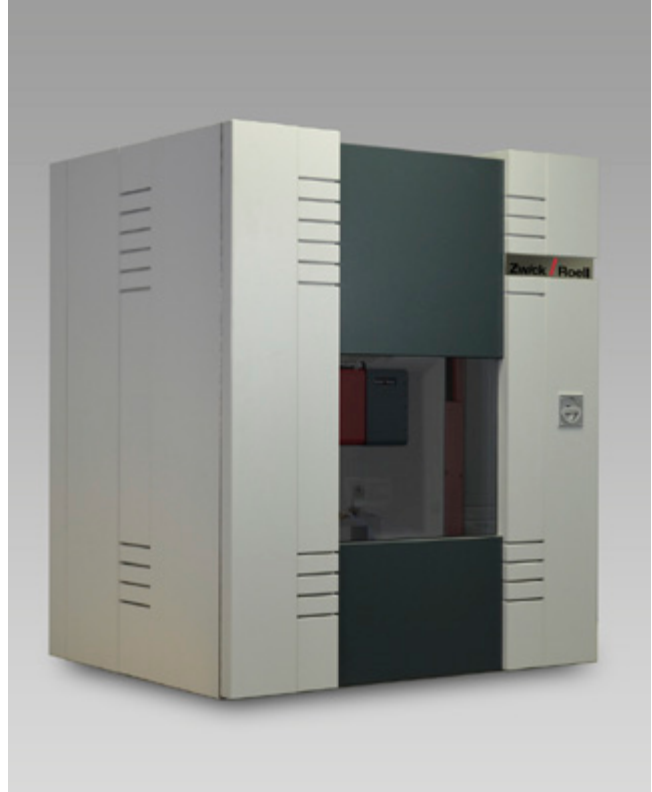
Fig. 2: ZHN with housing for thermic and accoustic isolation
